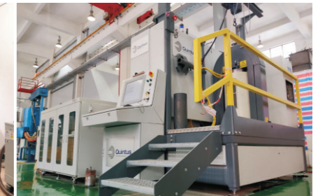
Hot isostatic pressing equipment
